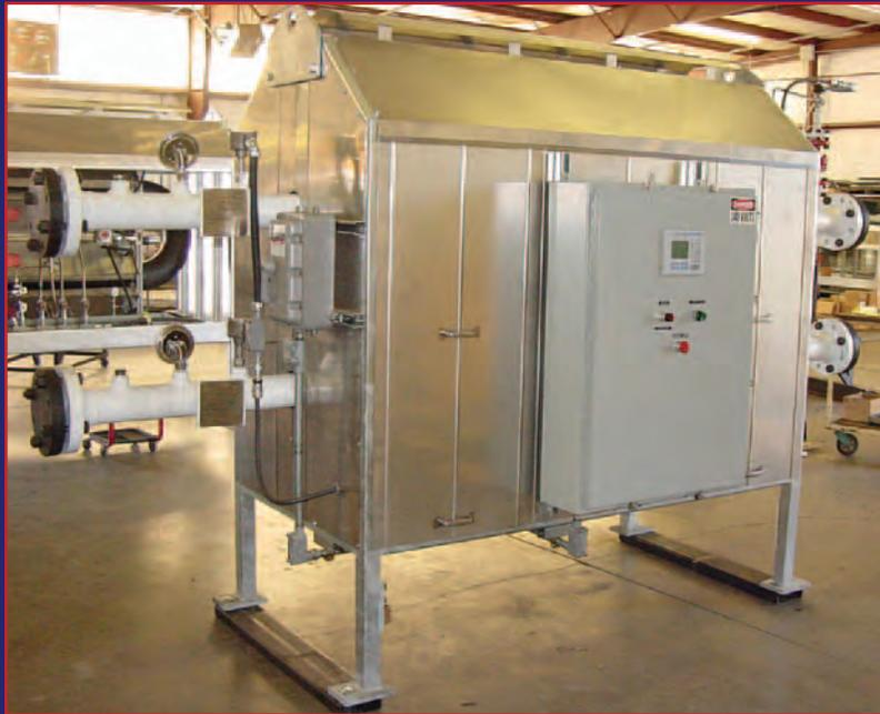
**Bruest HotCat is the most efficient technology available for long-term freeze protection of natural gas lines. The technology is also applicable for the heating of:**
